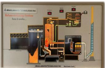
Hot combustion gasses pass by a series of boiler tubes filled with water, creating high-pressure steam. The steam is used to drive turbine generators and produce electricity for sale to local utilities. The steam also can be sold to drive industrial processes or for heating & cooling. The remaining steam is condensed into purified water and returned to the system for more renewable energy production.
